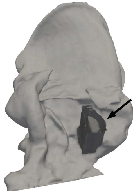
FIG. 2. Artificial ear canal (dark shading, arrow) attached to the right pinna in a rendering of a smoothed triangulated surface mesh.
